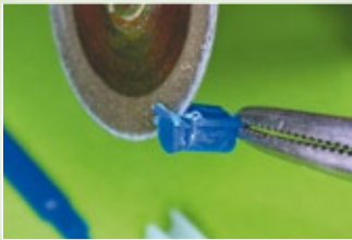
The attachment and the clip can be mounted with its original height (5 mm) or shortened (3.5 mm) by filing the side opposite the hole.
