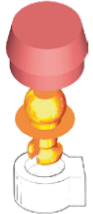
TOOL to hold the sphere
