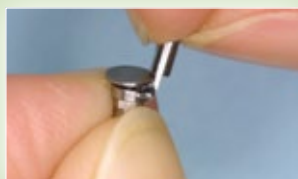
Bend the locking key and brake it.
