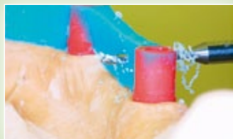
Model the bar in resin and drill a 0.8 mm hole in the most ideal position.
